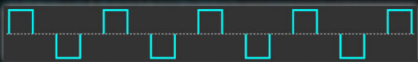
Modified Sine Wave: Harmful to devices
