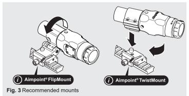
The height of the mount is correct when the optical axis of the 6XMag-1 and the Aimpoint sight coincide. Select a suitable position for the 6XMag-1 on the weapon base so the eye relief is correct and feels comfortable.
